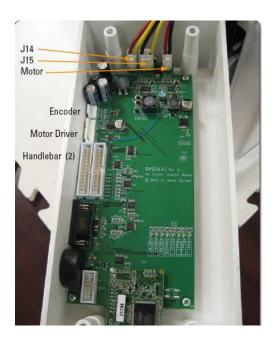
With the power turned on, use a volt meter measure the voltage on connector J14 and J15 on the 'C' pod.
