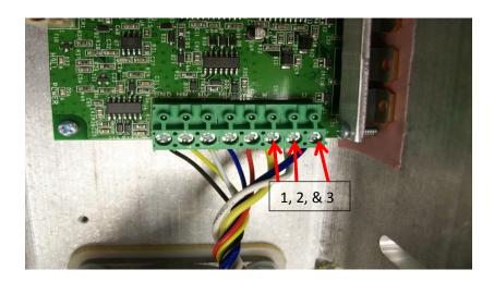
On the motor drive board, you should be getting 48 volts +- 3 volts from connector 'A'. If not, Replace the motor drive board
