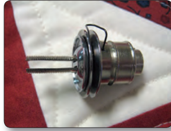
Figure 1.7 Detent washer and cone spring removed
