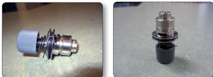
Figure 1.5. Top tension assembly, fully assembled (two views)
