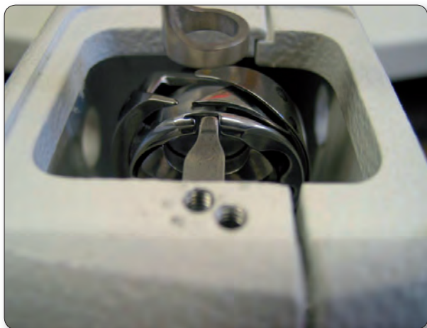
Figure 9.6 Stop-finger engaged without bobbin case
