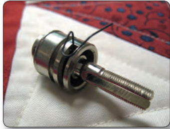
Figure 1.8 .Tension discs removed (two views)
