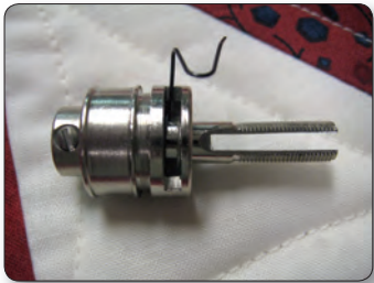
Figure 1.8 .Tension discs removed (two views)
