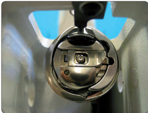
Figure 9.5 Stop-finger engaged with bobbin case installed
