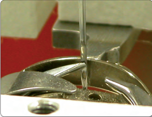
Figure 9.8 Loop lift and needle height both set correctly
