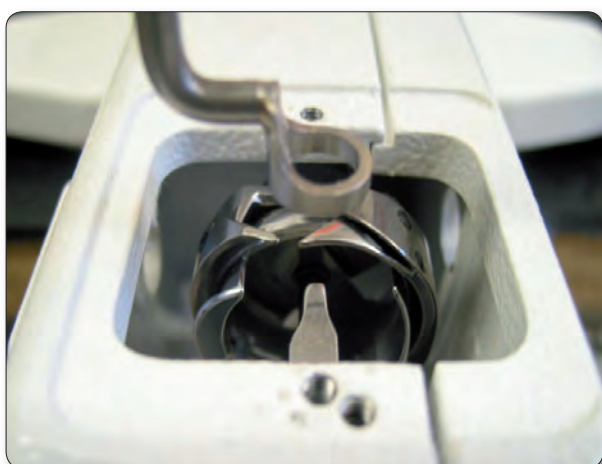
Figure 9.7 Basket rotated 180 degrees down, facilitating needle distance adjustment
