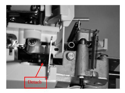
2. Detach the Shepard Hook from the Presser Foot Lever, in order to remove Roller Assembly from the machine.
