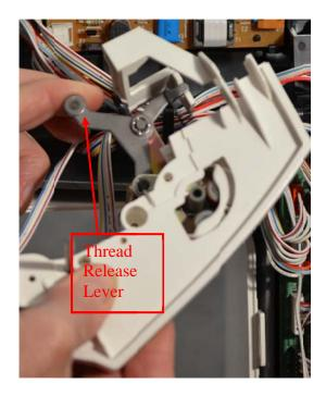
4. Pull down Thread Release Lever, to enable you to remove Thread Guide Cover.
