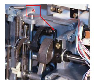
7. Reattach Shepards Hook "A" to Thread Release Lever, insure that Presser Foot is down
