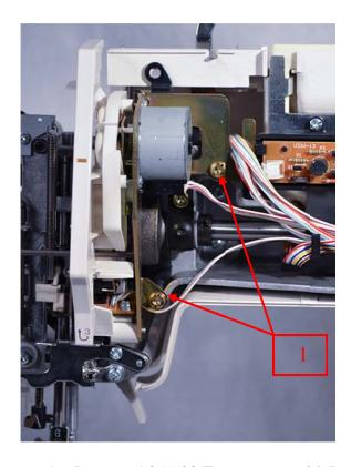
1. Remove '2 '#20 Torx screws with Presser Foot Lever in the down position.
