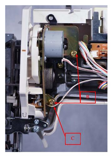
8. Attach ' 2 ' # 20 Torx screws " B " being careful that the Sensor Wire is routed ' C ' properly.
