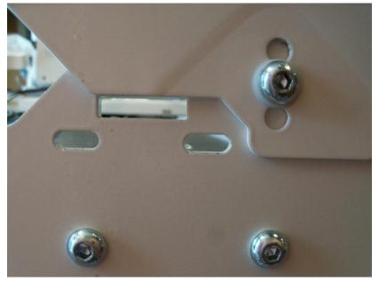
Attach the belt to the QuiltMotion Motor plate assembly, step 7 in QuiltMotion Instruction Manual. Follow the instructions in the manual to insure your belt is aligned correctly on the frame and the gearbox of the Motor Plate.
