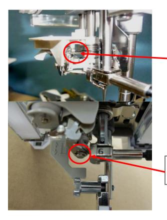
1. First detach spring from metal plate, with use of a small tool such as a crochet hook.
