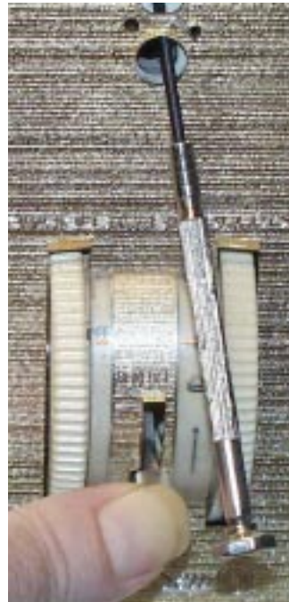
Zigzag Stitch, Right Needle Position, 21/2 Width Power Switch Off, Stitch length to 6, and Buttonhole dial in Off position.
