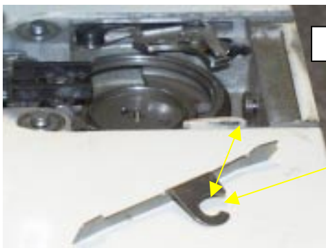
Place the horseshoe around the holding screw. Lift the plate onto the frame, and tighten the holding screw.
