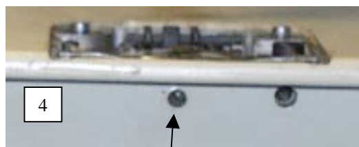
Loosen this screw, turn clockwise
