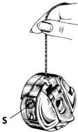
Fig. 30 Determining correct bobbin thread tension
