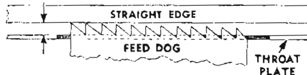
Fig. 11. Feed Dog at Correct Height
