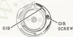
Fig. 38. Removal of Gib Screw and Gib
