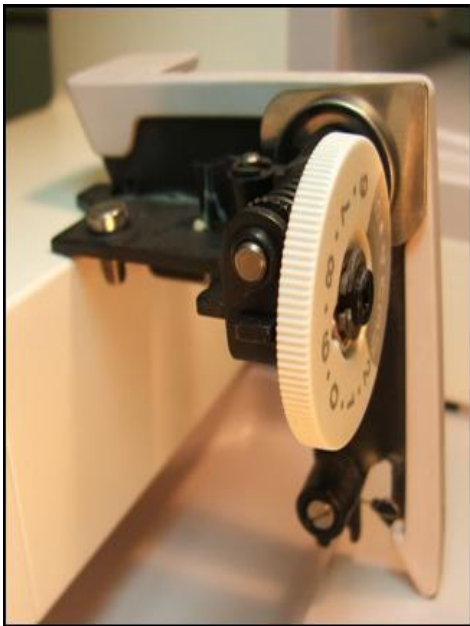
Tension unit after removal.
