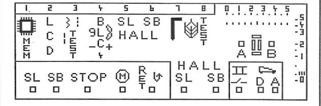
By means of the track-ball, bring the cursor over the required number or field, and select by pressing the OK button. By pressing the CLEAR button, you will always return to the basic menu of the service-programme, with the exception of the MEM-test and the LCD-test, which return automatically.
