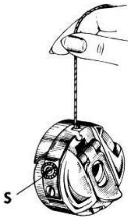
Fig. 30 Determining correct bobbin thread tension
