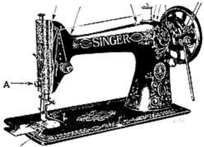
FIG. 17. FRONT VIEW, SHOWING OILING POINTS
