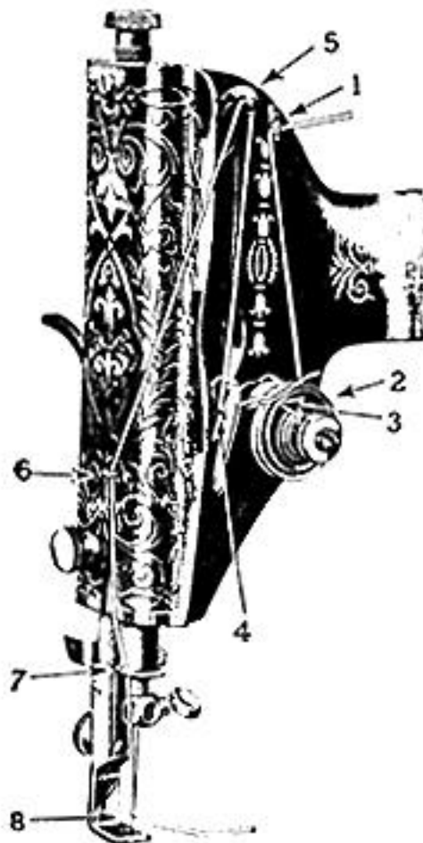
FIG. 11. THREADING THE NEEDLE
